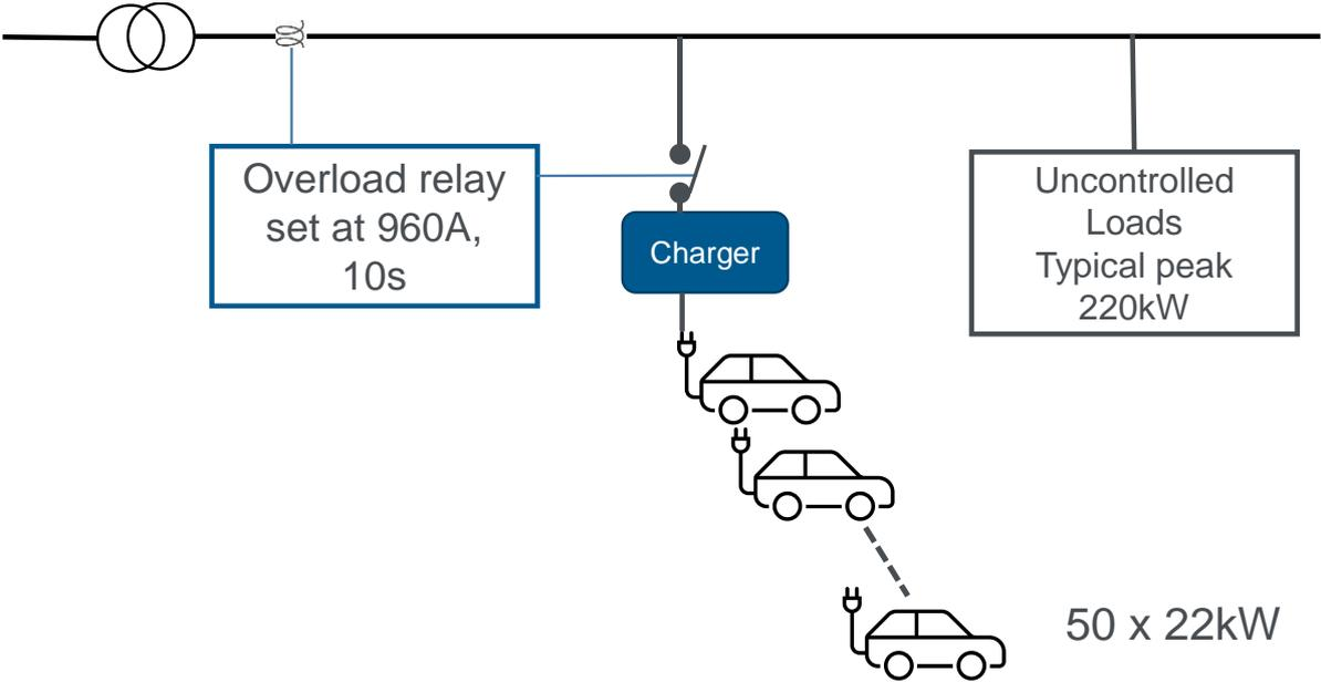
Figure E 7 Overload Protection Option (b)
