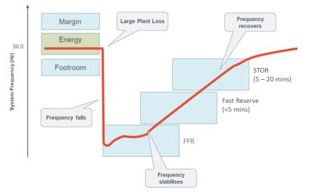
Figure 5: Timing of FFR, FR and STOR in response to large plant loss
