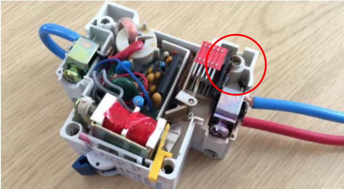
EV Charge point Contactor Normal Image
